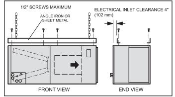
FIGURE 3. Suspending Horizontal Unit
