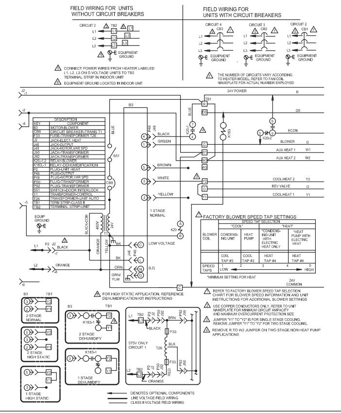
FIGURE 12. Typical System Wiring Diagram – 460V, Single- and Three-Phase Units (-036, -048 and -060 only)
