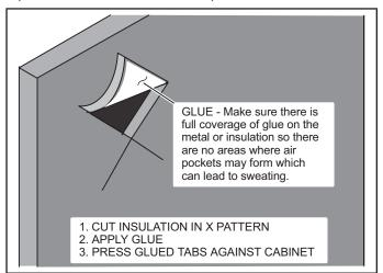
FIGURE 13. Repairing Insulation
