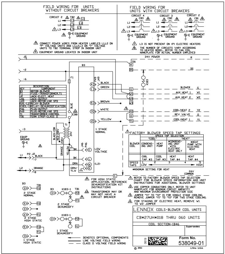
FIGURE 11. Typical System Wiring Diagram
