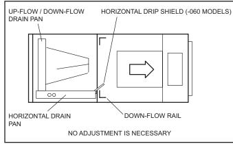
FIGURE 2. Right-Hand Discharge Configuration
