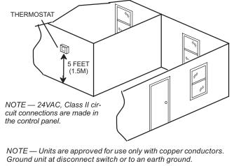
FIGURE 10. Thermostat Installation
